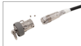
Pull the terminal over the line and fold the core of the line over the wedges. Insert the wedges to the terminal.
